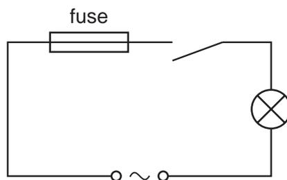
When the switch is closed the fuse blows and stops the current.
